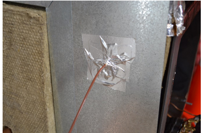
Other thermocouples attached to pipework. Thermocouple in heater to check temperature inside heater was constant.
