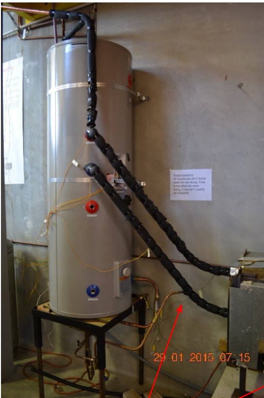
Rheem double coil, comparing rising and falling return pipe.
