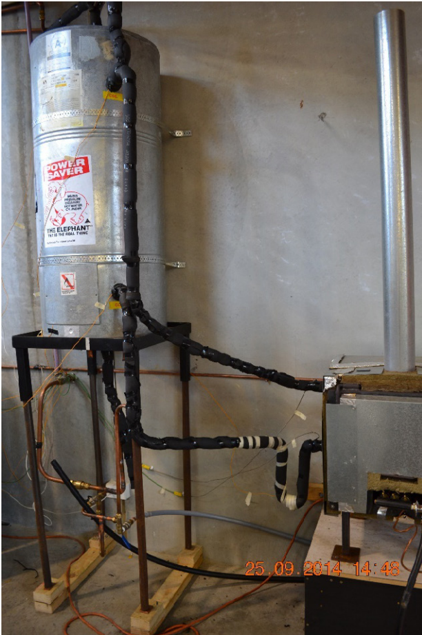
Elephant indirect with heat trap, flow and return connected to coil, conventional.
