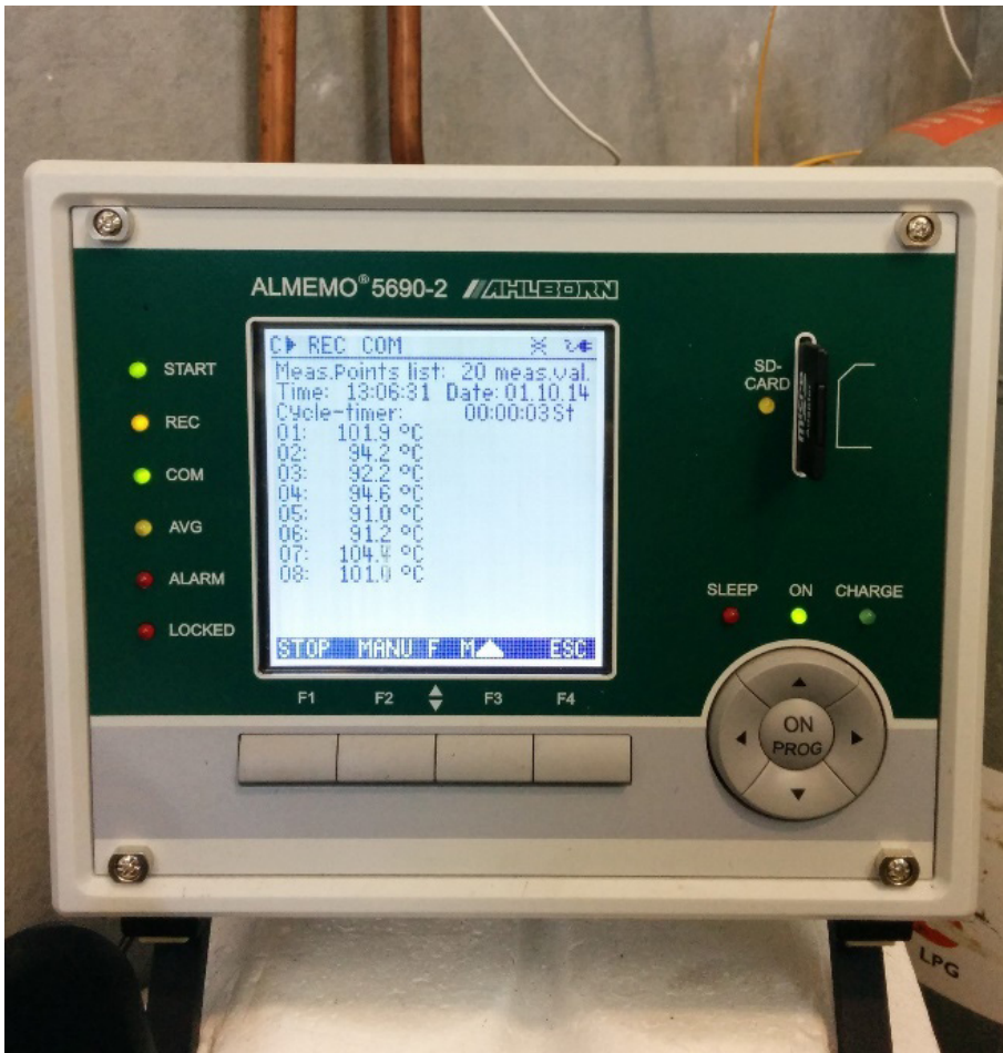
Data logger showing temperatures at all sensors.
