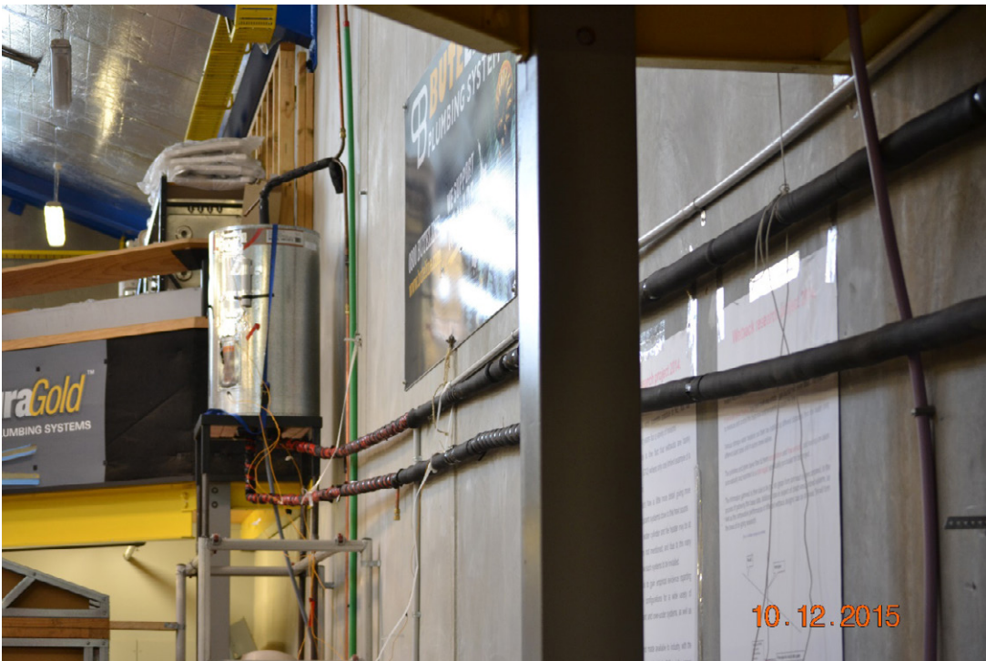
Wetback pipes at 10 m distance, conventional connections.
