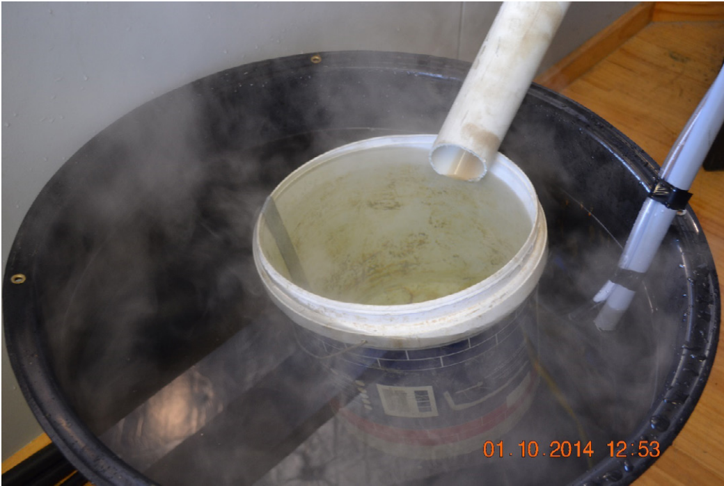
Boiling water discharged through vent pipe being captured and measured.
